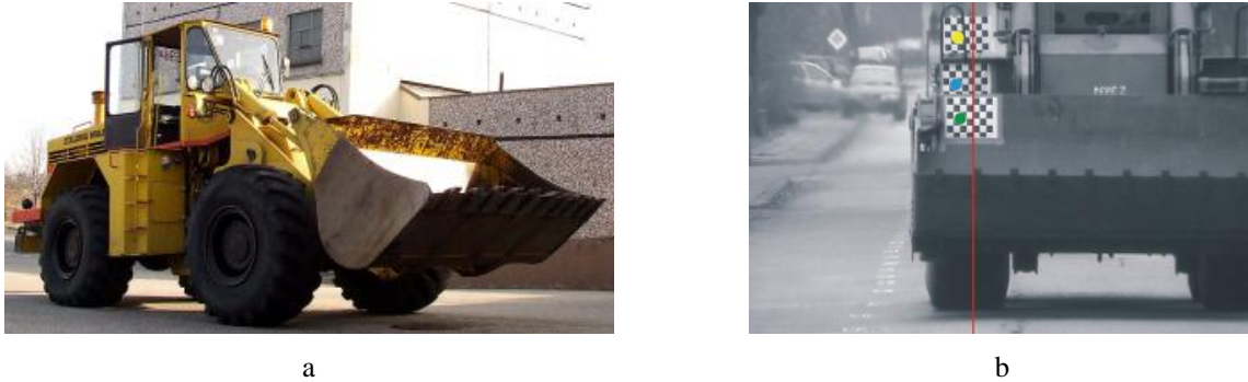
Fig.2. The SL-34 loader: a – general view; b – on trial track during test
