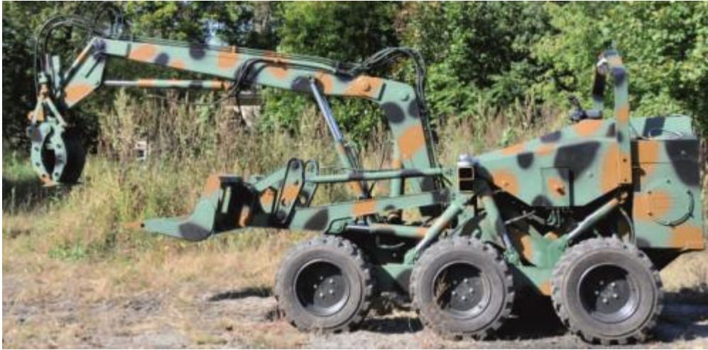
Fig. 2. Unmanned Ground Vehicle MAREK with 6x6 drive system and skid steer
