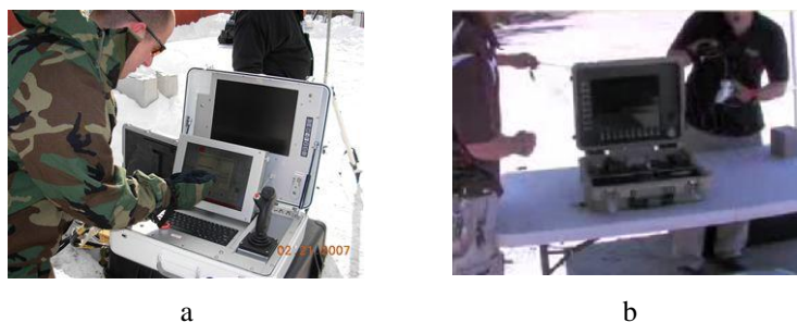
Fig. 1. Different control panels for unmanned engineering equipment: a – All All-purpose Remote Transport System's control panel (ARTS); b – Bobcat's Robotic Controller Kit's control panel
